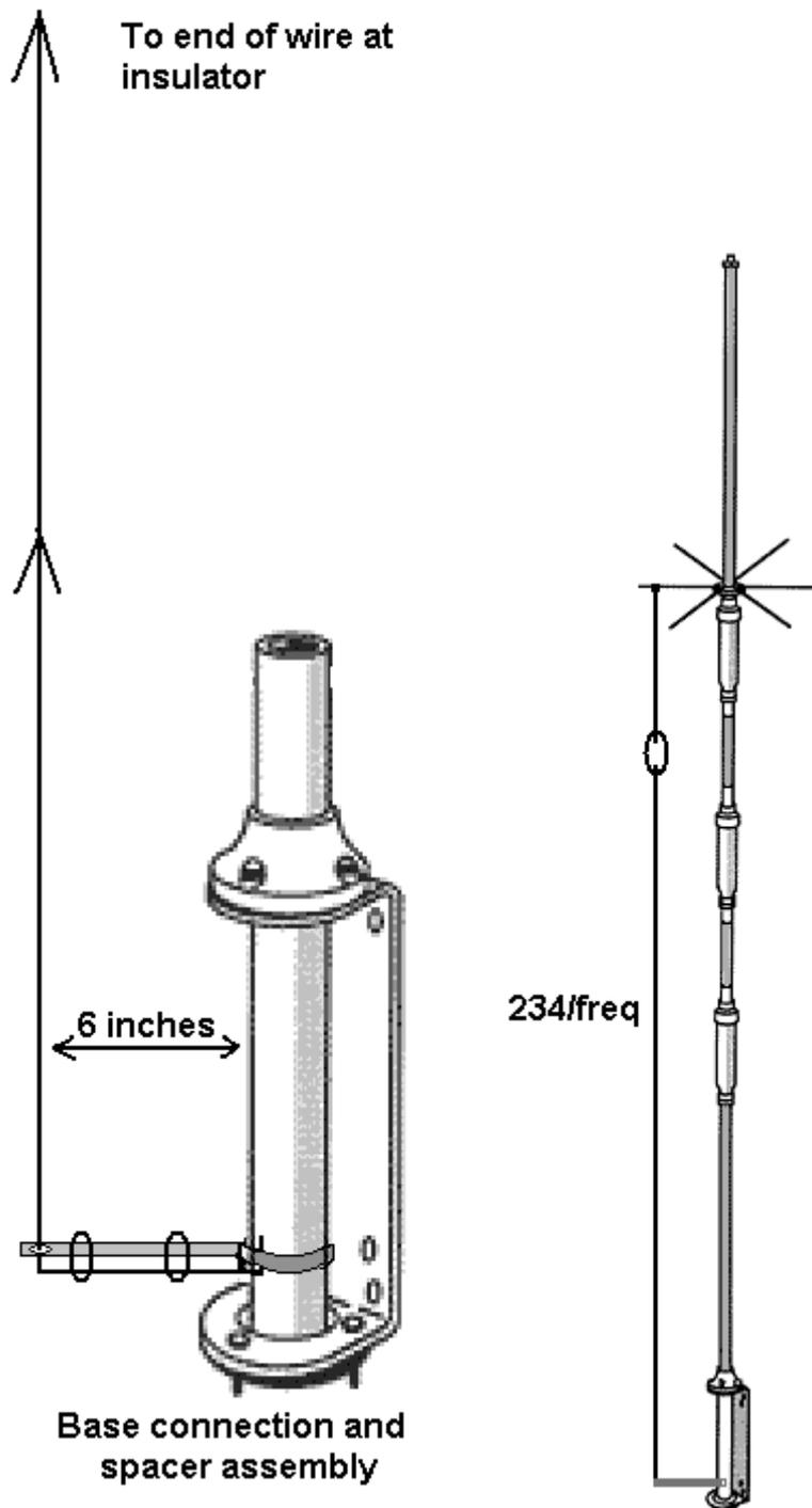
**NOTES:** In drawing above left, the 2 ovals near the bottom do not represent coax shield. They represent nylon wire ties to secure the wire to the aluminum bracket.
