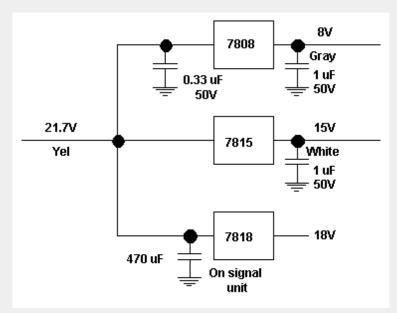
The regulators need capacitors near them, especially if they are driving the PIEXX board, which has switching regulators with inductors at the input. The regulators should be prewired, and the wires are connected to the voltage points inside the power supply fan case.
