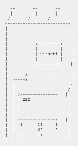
The X's are where the 100uF capacitor is soldered to the board. Just tack your wire onto the capacitor's negative lead or onto it's circuit pad.
