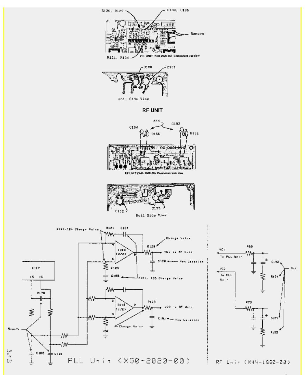
In some TS-940S below S/N 711xxxx, a "popping" or "clicking" noise may be heard when the squelch circuit is opened or closed. This may be more noticeable when an optional CW filter is installed. The following procedure will minimize the noise.
