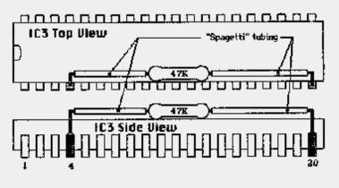
Solder the 47 Kohm resistor directly to pins 4 and 20 of IC13. Don't overheat or use too much solder. You must use an iron with vltage isolation on the tip!.
