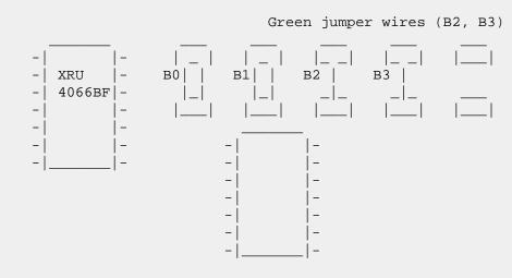
The jumpers are actually soldered on the other side of the board, but the loops come up over the top and hang over the B0/B1 side.
