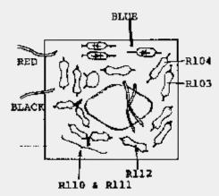
procedure for replacing the resistors in the HET unit is to first remove the three screws holding the board and tilt it up towards the VFO. Plugs P-1 and P-2 may be removed if necessary. The resistots that need to be changed are located on the outside edge of the board. Replace the resistors and reinstall the board and connectore. Install the crystals in the sppropriate sockets (X3, X4, and X6). Replace the FINAL tuning shaft and align as per page 40 of the Service Manual.
