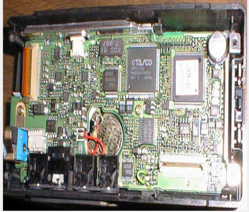
9. Locate the green wire. Under the green wire there are four small diodes in a neat row (they should have a miniature A on them if your eyesight is good). Using a soldering iron, remove the middle two diodes.
