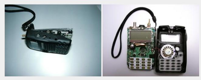
8. With the radio opened up like a book, look at the left hand side of the PCB just to the left of the PCB mounted microphone. You should see two diodes and also a open pad just below were another diode could be fitted.
