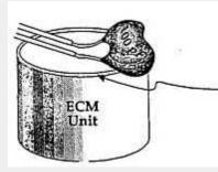
Make sure the leads of C8 100 pF capacitor do not touch the ECM case.
