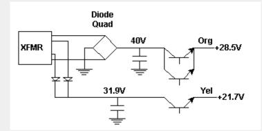
The power switch has a pole that opens the +28.5V to most of the radio, including the circuit that runs the 21.7V regulator. This is apparently so the radio will just turn off without the time delay and rude noises of the filter capacitors discharging.
