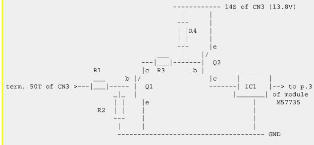
R1 + R2 + Q1 = DTC114 or R1= 10k, R2= 10k, Q1= BC547 (NPN, Ic max= 100mA)
