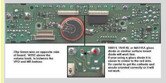
1N914, 1N4148, or MA141A glass diode or similiar surface mount diode will work fine.
