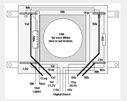
Cut to length and solder the Yellow, Black, Gray and White wires to the terminal strips, making sure they are connected to the same color wire that is already there. Dress the wires in place to avoid the fan with a tiny nonmetallic cable tie or twister.
