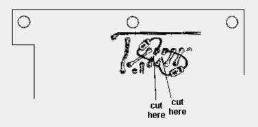
The foil paths from the connector to diodes D18 and D19 are cut and the new diodes soldered on the foil side of the board. The cathode and of the diodes is soldered to the connector side. We recommend using either 1S2076 or 1S1555 diodes.
