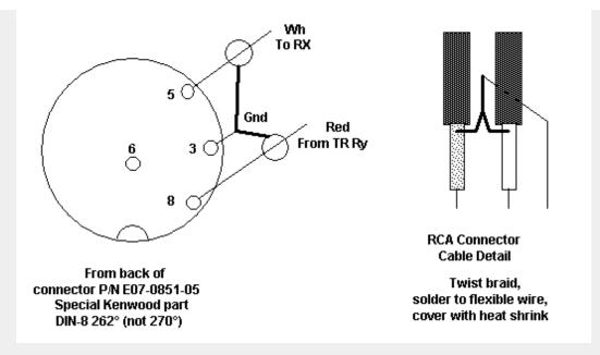
It's good practice to have a relay that disconnects the receiver input from any antenna and shorts it to ground during transmit, so the transmit power isn't returned to the receiver from a separate receiving antenna. When used as a second receiver in a multi-op setup, this relay can also be run by the AMP relay line of the transmitter on the same band.
