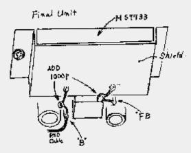
2. On the RX unit X55-1270-10 add three additional 1000pF caps (c52-1710-26) and one additional 470pF cap (C52-1747-16) as shown.
