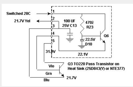
Use an insulated clip probe. If the output of the 21.7V supply measures OK on the yellow wire at the terminal strips in the power supply fan case or the black terminal strip in the narrow space between the output low-pass filter and the antenna tuner, then all is OK.
