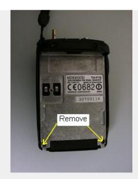
7. To open your radio's case. It's best to gently open the radio from the bottom until you have a gap of about 10mm. Then hold the front panel in the palm of your left hand and gently slide the main body of the radio downwards with your right hand, until the aerial and frequency change encoder shaft are clear of the holes in the top panel of the radio. Take care not to open the radio to fast, because the internal speaker wires are very short.
