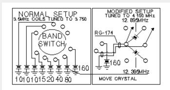
The modification consists of moving the 12.395 MHz crystal from the Band Switch to a small DPDT toggle switch mounted on the bottom of the case. An additional 12.895 MHz crystal is added to the switch for the new range needed.
