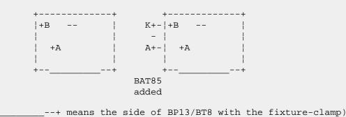
+B means the battery-plus, +A the accu-plus -- is the common grond (accu- and battery minus.)
