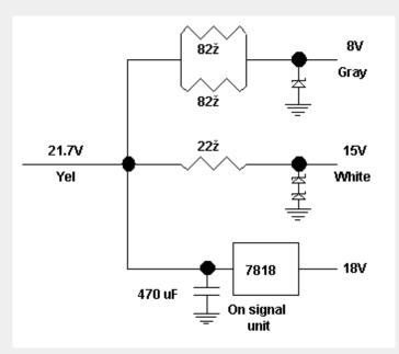
The main schematic diagram of the radio is wrong, it shows the 33? resistor that is the third supply voltage for the digital board connected to the 21.7V instead of the 28.5V line.
